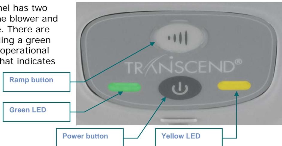
1. Connect the Transcend to a power source and allow it to enter Standby Mode.
